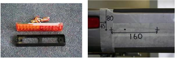
2. Mark bumper as per photo. Drill two outer holes to 6mm and hole for wiring to 10mm. About 50mm in from screw holes.
