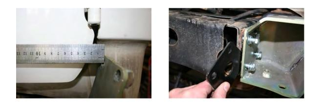
Slide the flat plate with 4 10mm nuts welded to it into the chassis (Note which way it goes in to align the four holes in the side of the chassis) and fit the four 10mm bolts through the chassis into the plate.
