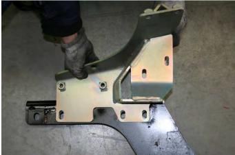
Remove the original chassis side bracket ('U' bracket). This is the bracket which supported the metal bumper
